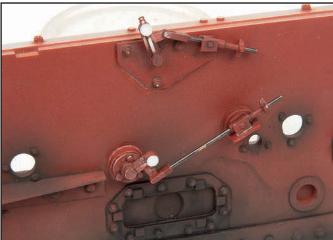
The upper adjuster plate was glued in place on the rear wall after much testing and having removed the upper tensioning wheel so that I could add new shafts to bridge the gap between each adjuster and its wheel. Note the damage caused to the paintwork through these adjustments.
