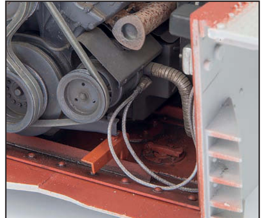
The collar was glued in position onto the output socket of the dynamo.
