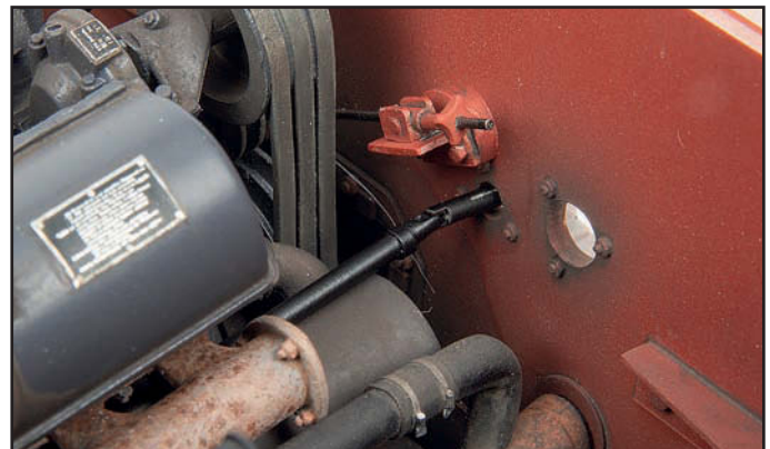
The rear plate was dry fitted again and the other half of the joint test fitted through the starter port, successfully!
