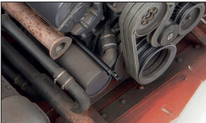
The shaft had been shortened to accommodate the universal joint and was refitted onto the starter motor.
